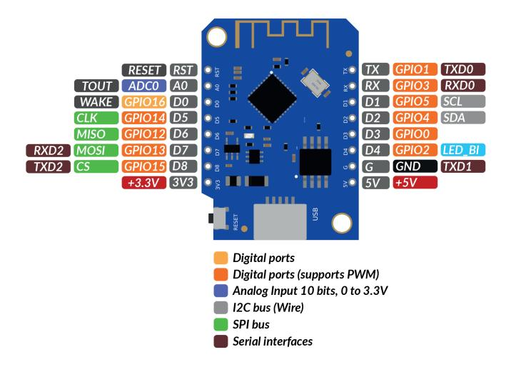
Note: The D1 Mini V3 module has a 5V voltage output pin to power the external electronic devices connected to it, but it is not 5V tolerant! The 5V pin is power output pin, which outputs power from the microUSB port.
